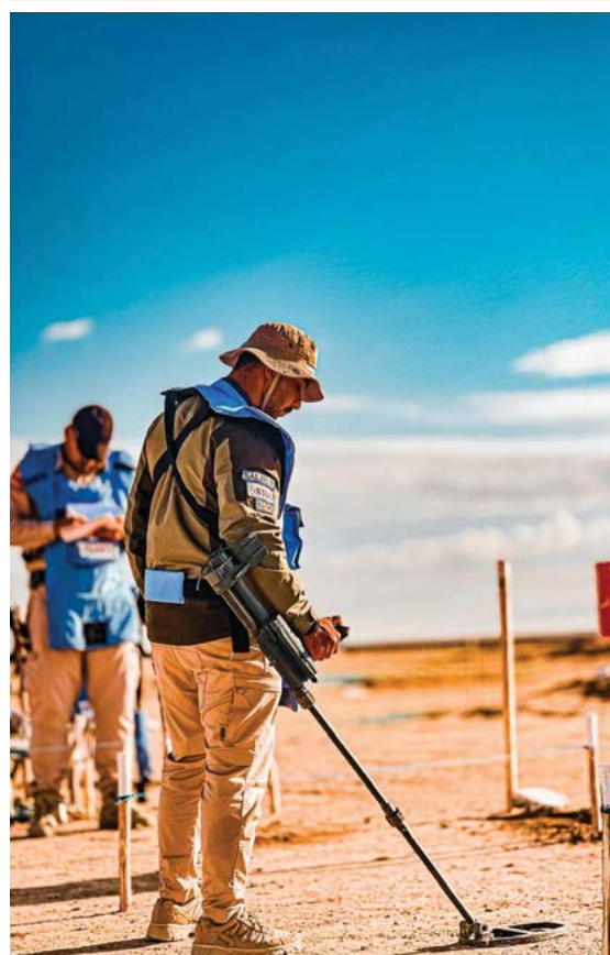
A deminer performs a daily check of his metal detector in a safe, testing area before starting clearance operations in Tal Afar, in Iraq's Ninewa governorate.
